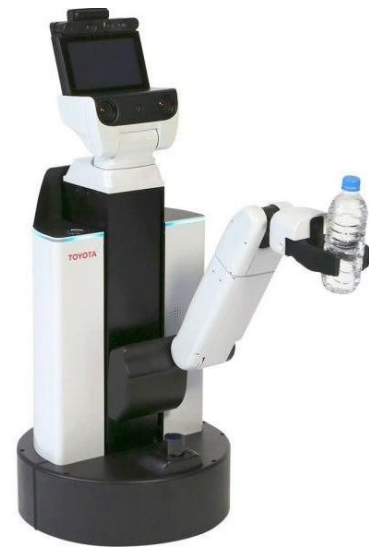
Toyota HSR Cost: not commercially available Footprint Width: 43cm (17") Weight: 37 kg (82 lb)
