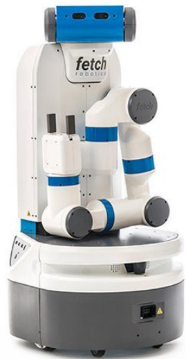
Fetch Cost: ~$100,000 Footprint Width: 51cm (20") Weight: 113 kg (250 lb)
