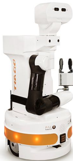
PAL Tiago Cost: $58,485 (base model) Footprint Width: 54cm (21") Weight: 70 kg (154 lb)
